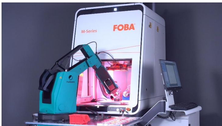
Automatic loading and unloading of a laser marking machine using the robot system from fruitcore. (Image rights: FOBA)
